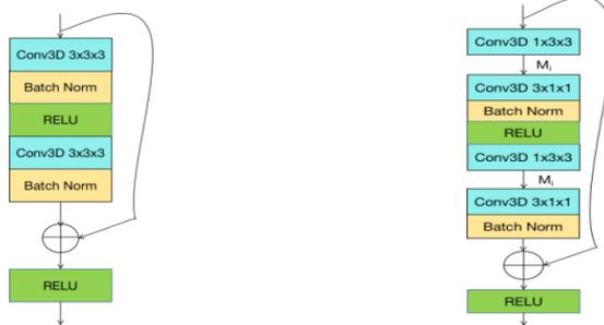
Figure 4. R3D block vs R(2+1)D block a) The residual building-block used in the R3D architecture. b) The residual building-block used in the R(2+1)D architecture.
